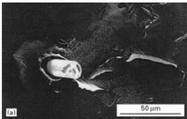
Figure 6 Upper and lower fracture surfaces associated with the arrest line around the glass fibre during crack growth of Fig. 4.
